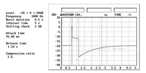
Fig. 4: Example of a display obtained with the measurement program
