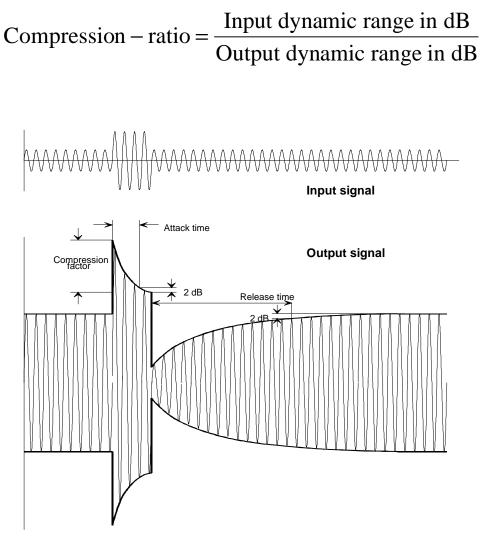
Fig. 1: Response of an AGC circuit
