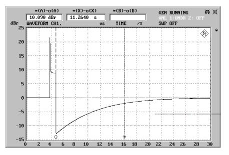
Fig. 3: Example for manual determination of the release time
